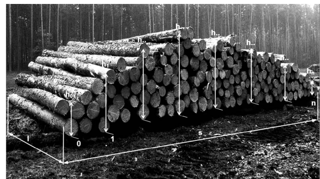
Figure 1. Elements of irregular stack measurement ( h 0 – h n – height, l – stack length, s – stack width) (Witkowska, Jodłowski 2018)
