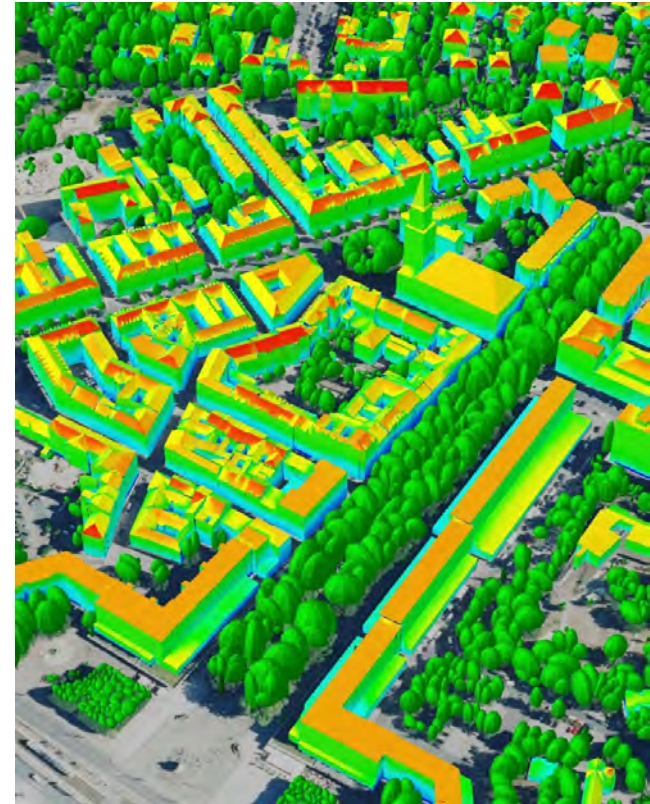
Visualization of solar irradiation in the 3D city model: Innere Neustadt Dresden. (© TUM, Chair of Geoinformatics, 2022)
